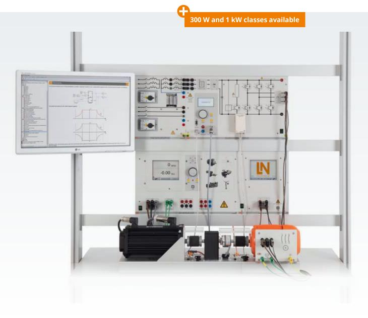
Three-phase drives are used today in almost all electrical drives. Mathematically the automatic control of such drives is both a complex and costly undertaking. The training system makes it possible to simulate sophisticated control algorithms with the aid of the special toolbox for Matlab®/ Simulink® and subsequently test them by means of automatically generated code on real intrinsically safe hardware incorporating a motor and load.
