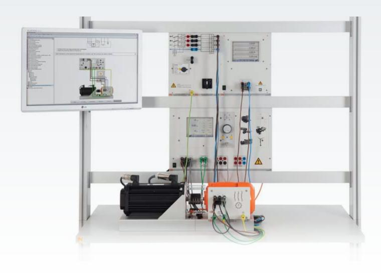
Reluctance motors are a mixture of asynchronous and synchronous motor. Thanks to the special rotor design with salient poles, the motor can start like an asynchronous motor. After a certain speed is reached, the rotor runs synchronously with the stator field. Reluctance machines are used for example in the textile industry for the synchronous de-spooling of yarn. This entails several motors being controlled by one frequency converter.
