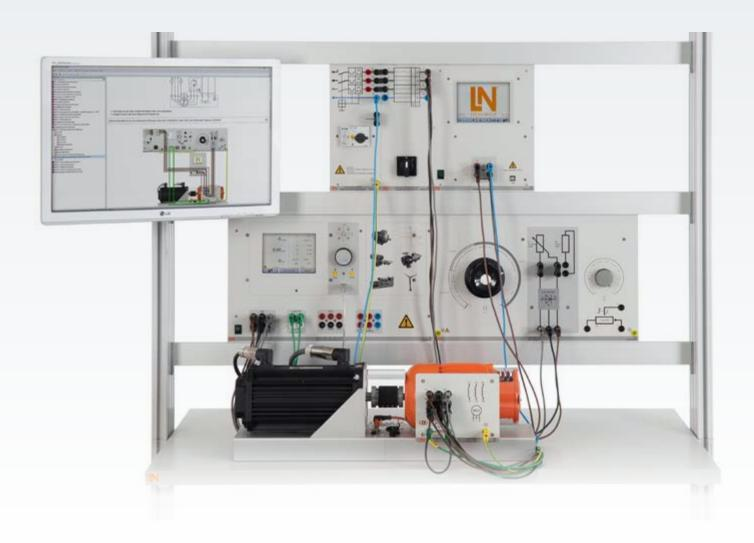
In contrast to squirrel-cage rotors, slip-ring rotors have a rotor equipped with wound coils. These can be connected to resistors or static converters via slip-rings. Speed adjustment is performed via these connection terminals.
