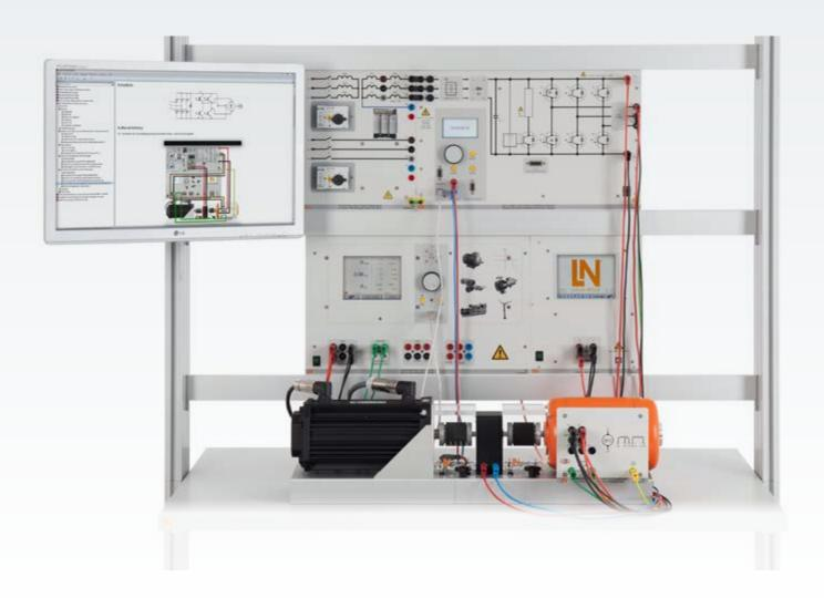
Thanks to their simple control structure, inverter-fed drives with DC motors are ideally suited to serve as an introduction to the subject of speed-variable drives. By considering closed-loop current control and speed control separately, students are able to put the controller into operation and optimize it step-by-step. The training system graphically demonstrates how a speed-variable system operates.
