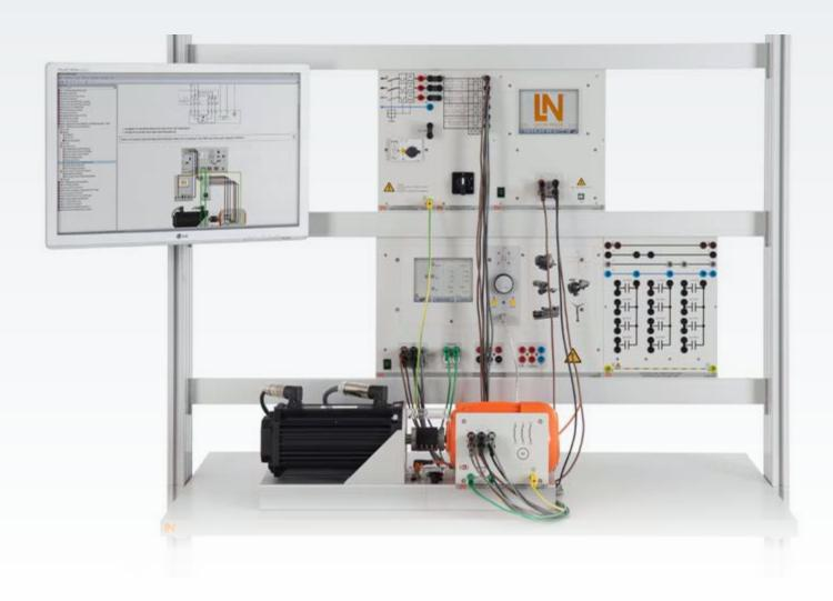
Three-phase motors with squirrel-cage rotors are the most frequently used in industry. The maintenance-free and rugged motors can be manufactured cost-efficiently. These motors can be found ranging from low power levels in the watt range up to power levels of several megawatts. Thanks to the use of modern frequency converter technology, these motors can vary their speeds virtually loss-free so that there appears to be no end to new application areas for these motors.
