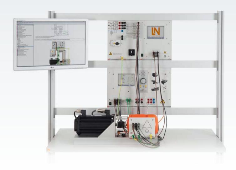
Thanks to its special winding, the three-phase motor with Dahlender circuit is able to operate the motor with squirrel-cage rotor at two different speeds. The ratio of speeds is 2:1 for this circuit. With this motor type, simple drives can be designed with two speeds, for example, a two-staged ventilator drive.
