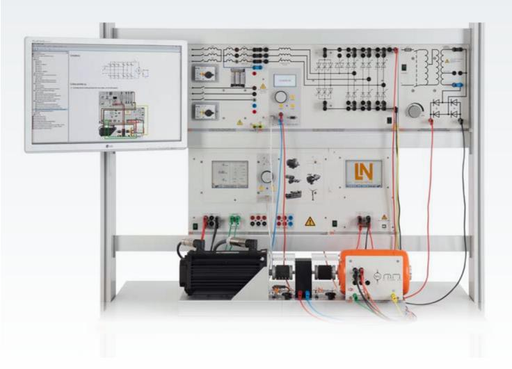
Variable-speed DC drives excel thanks to their very good speed and torque controllability and extremely high dynamic response. When it comes to power semiconductors operating with large-scale drives at high power levels, one resorts to line-commutated converters with thyristors. These components stand out because of their capacity to handle overload and their low tendency for power losses.
