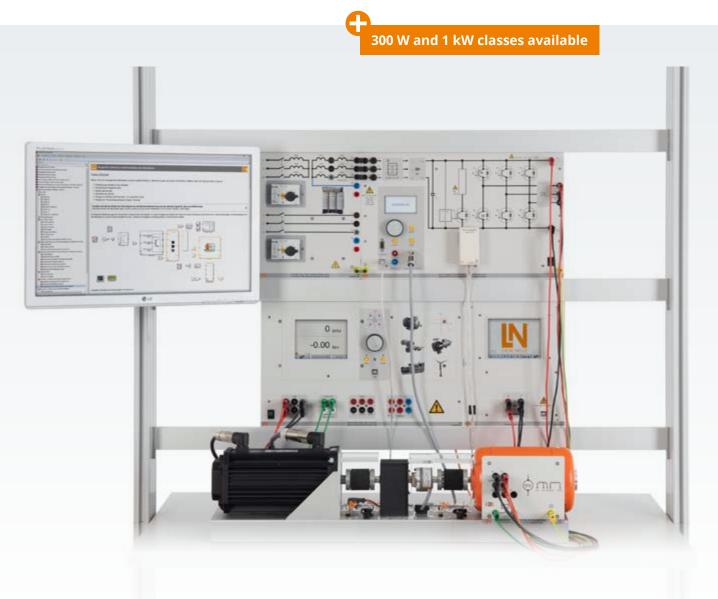
Thanks to their clearly arranged control structure, converters with DC motors are particularly well suited for programming your very own initial control algorithms. The training system permits implementation, optimization and operation of your own control configurations. In addition to classic approaches, this open system enables you to also safely explore new ideas and novel expansions.
