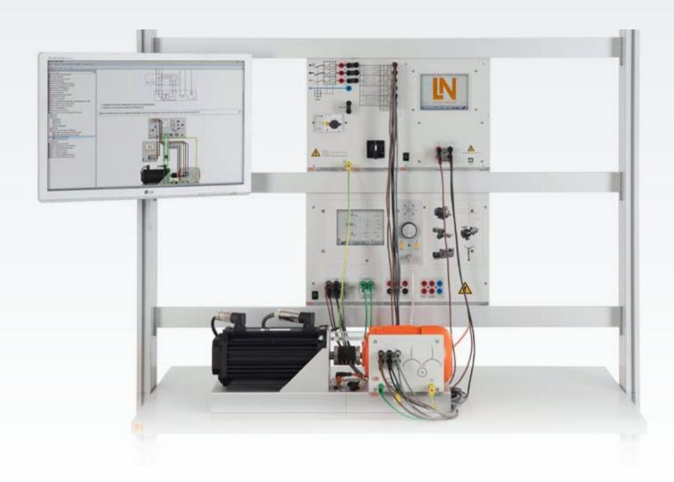
The system consists of two three-phase motors in a single housing with separate windings. Since both windings operate separately from each other, different integer ratios can be produced between the speeds. The motor is used for simple applications wherever the ratio between slower and faster speed is greater than two, for example in crane applications with creep speed and high speed.
