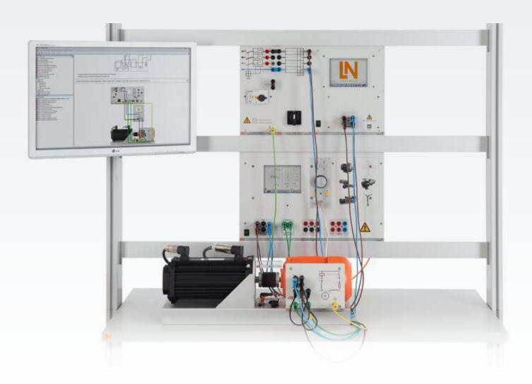
Single-phase motors with bifilar starter winding are asynchronous (induction) machines. Besides a primary winding, they have a starter winding with high internal resistance, which is partially bifilar designed and thus magnetically ineffective. It is disabled after start-up. The motors do not contain any parts which are subject to wear and tear such as collectors or slip-rings and operate with fixed, almost synchronous speed. The power range can reach up to around 2 kW..
