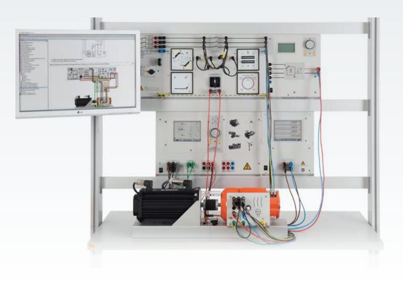
In mains synchronization, the unloaded generator is connected to the mains power grid. Voltage, frequency and phase-angle have to coincide with the corresponding variable on the mains power grid. To measure these variables, a variety of different measuring instruments are used. The variables are set by means of the generator speed and generator excitation.
