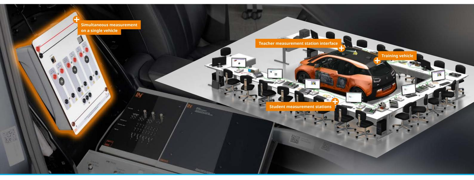
The measurement expansion package permits multiple trainees to conduct measurements and perform diagnostics at the same time on just one vehicle thanks to the inclusion of the student measurement stations.
