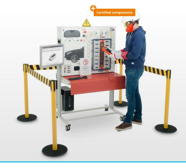
Working directly on a real high-voltage battery and inside it: The system is set up to be just like a high-voltage battery in a standard production vehicle. With this training system, trainees can make measurements and diagnoses inside the high-voltage battery, working down to the level of individual cells and even replacing them.
