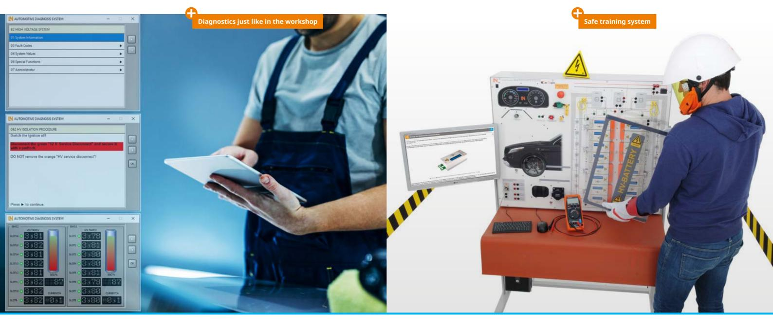
The built-in diagnostic tester makes it possible to train and learn diagnostic procedures as used in real vehicle workshops.
